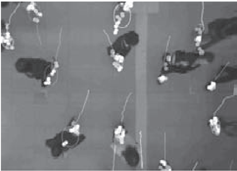
FIGURE 4.9 A back-projection of laser points onto a video image, where the spatial resolution was about 0.38 \text{ person}/m^2 .
