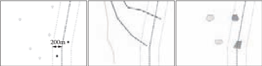
FIGURE 1.4 Distance search operations for (a) points, (b) line segments, and (c) polygons, part of which are within 200 meters from a given line indicated (the dot–dash lines).
