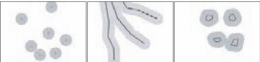
FIGURE 1.6 Buffer operations for (a) points, (b) line segments, and (c) polygons.
